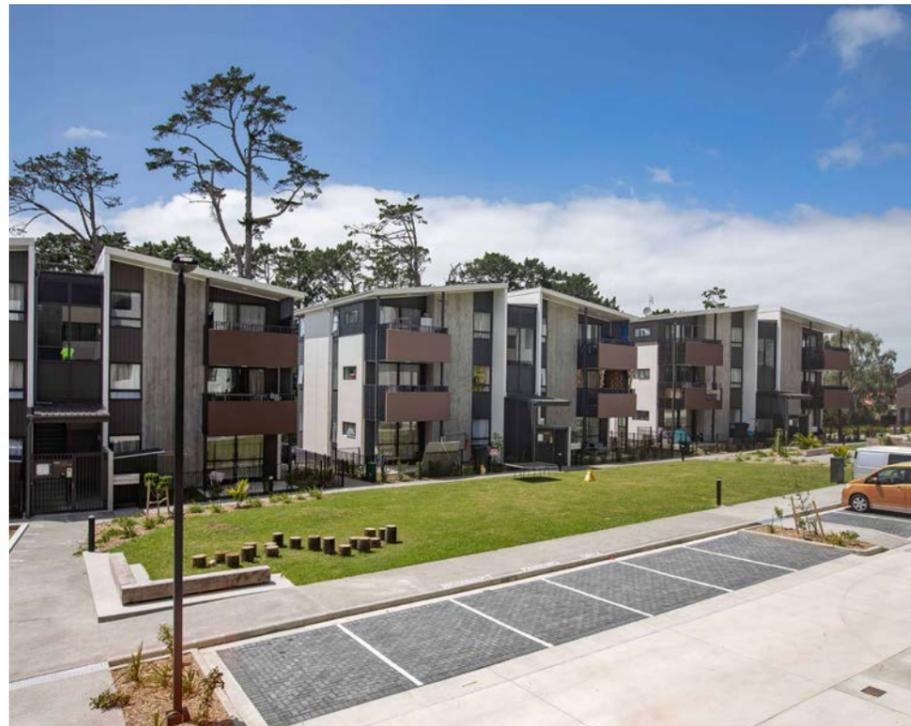
Consider changes in surface material that differentiate parking bays from manoeuvring aisles, to break down the visual impact of expansive areas of hardstand.
