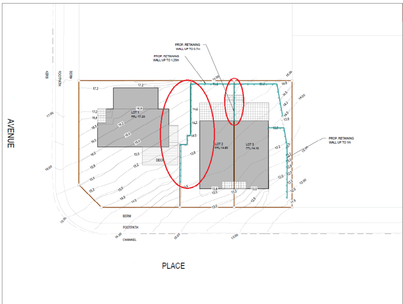
Figure 4: Retaining walls on the boundary within Kāinga Ora development (red circles)
