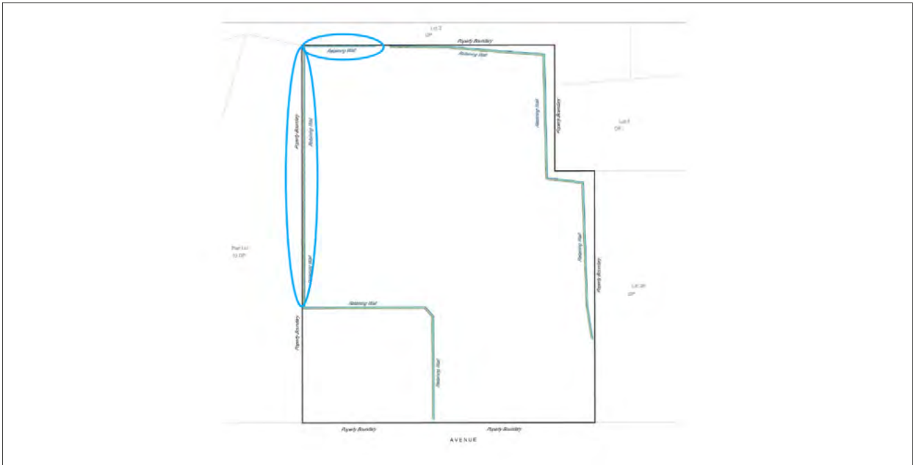
Figure 5: Retaining walls on the boundary shared with adjoining properties (blue circles)
